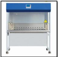
Safety Centrifuge Cups and Biosafety Cabinets (BSC) are the most common engineering controls used for the manipulation of blood and body fluids.
