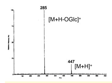
The *m/z* 285 ion results from collision events in the interface
