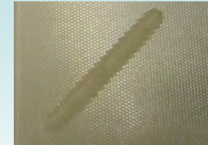
Weld of transparent textured polymer film (0.4 mm thick)
