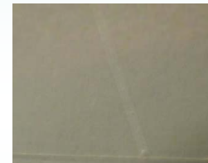
Weld of transparent PET film (0.1 mm thick)
