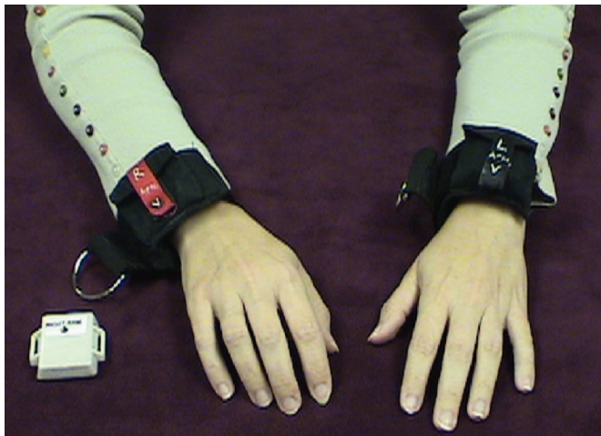
Figure. The accelerometers were placed in snug pouches sewn onto cloth and elastic bands, and one monitor was strapped onto each wrist. Participants wore the monitors for 3 days during all waking hours, except when they were in contact with water. The accelerometers (see unit next to right hand) contain a single piezoelectric crystal mounted in such a way that the monitors are sensitive to movement in two directions. The charge produced by the piezoelectric crystal when it is subject to acceleration is sampled at 10 Hz and integrated over a user-specified epoch. The integrated value, called a raw count, represents a rough index of the amount of movement by the object to which the accelerometer is attached. For example, lifting a can from a table to a shelf produces roughly 20 raw counts/second from a wrist-mounted accelerometer. The recording epoch in this study was 2 seconds; recording capacity for these wireless, self-contained monitors was approximately 72 hours.
