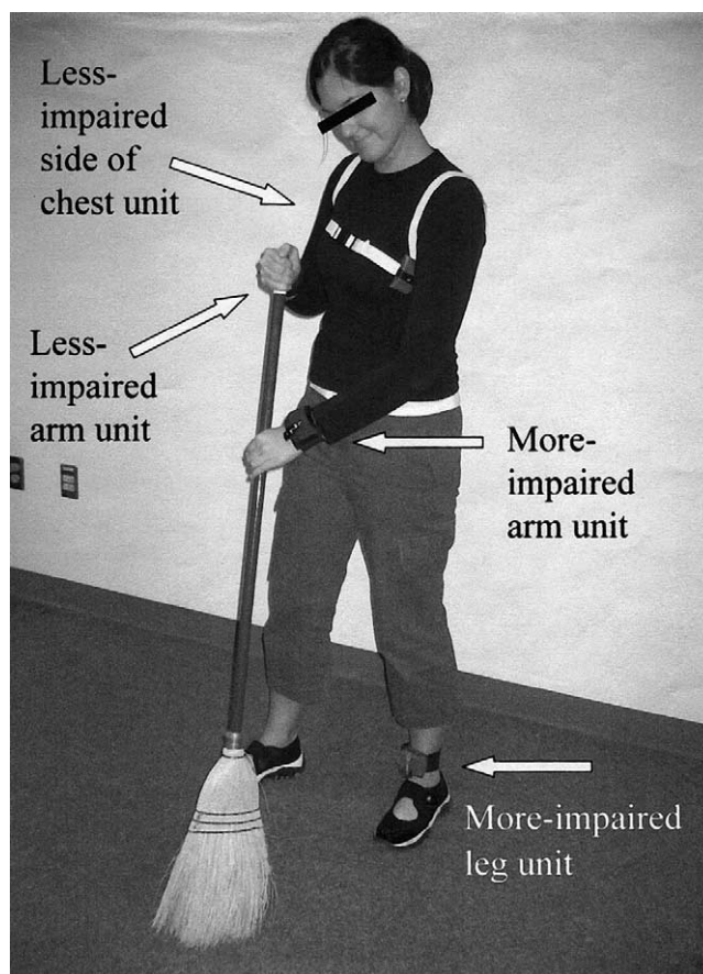
Fig 1. Accelerometer configuration. Four accelerometers were placed in snug pouches sewn onto terrycloth and elastic bands, and 1 unit was strapped onto each wrist, the chest (less impaired side), and ankle (more impaired side). Accelerometers were worn on both arms because a single unit worn on the more-impaired wrist might act as a cue to use that extremity and thereby confound the measurement of the effects of rehabilitation on arm function. In addition, recordings gathered from the less-impaired arm might serve as a comparison for data gathered from the more-impaired arm. The chest and ankle placements were chosen because examining the effects of rehabilitation on more-impaired arm movement that is independent of torso and ambulatory movements was thought to be valuable.
