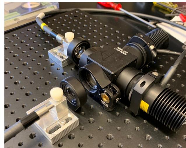
LEDs emitting at 500nm and/or 560nm are combined and transmitted through fiber optic cables to two targets. (440nm and 660nm LED can be interchanged)
