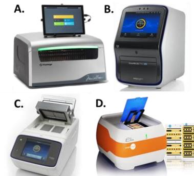
Figure 4. Equipment- Pandemic Preparedness Core. A. ProMega Maxwell RSC 48 Nucleic Acid Extraction System. B. Applied Biosystems QuantStudio 7 Dx Pro RT-PCR. C. ABS ProFlex PCR. D. Biotechne Protein Simple Ella Next Generation ELISA system.
