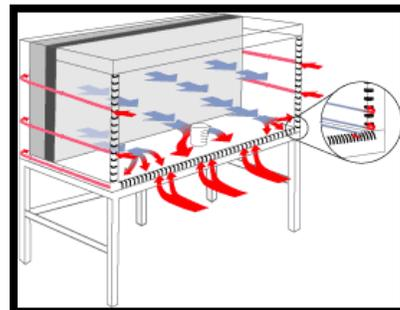
The bench provides product protection by ensuring that the work in the bench is exposed only to HEPA-filtered air.
