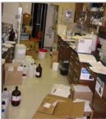
Floors should be clear of clutter to prevent accidents and provide a path in case of an emergency, especially a fire. This example is not only a fire hazard but a chemical one, as well.
