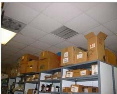
These items are stored too close to the ceiling. In an area without a sprinkler system, the fire code states that there must be a 24-inch clearance between the ceiling and stored items.
