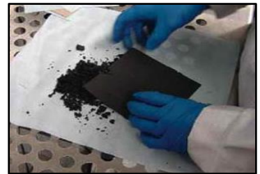
Shown here is crumbling carbon nanofiber paper on wet paper.
