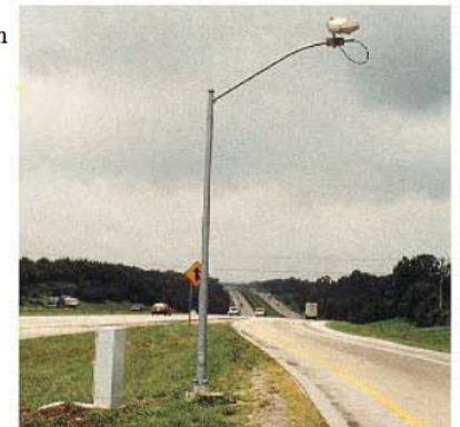
An exit AVI reader in Laurel County, Ky., identifies trucks as they leave the weigh station and records weight data on their transponders.
