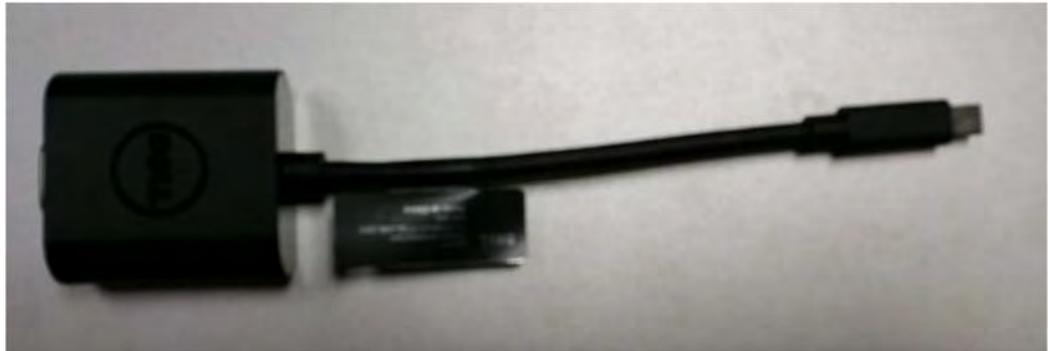
Connect the **VGA cable first**, then connect the adapter to the laptop. Once you have this adapter connected to your laptop and the VGA cable connected to the other end. Follow the steps in **Option 2** for VGA connections.
