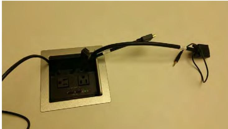
Each HDMI cable has been labeled. Plug one of the HDMI cables into your laptop's HDMI port and take note of the cable's label. Refer to the panel instructions to switch the TV to your laptop's video connection. (If you used the cable labeled "HDMI 1" you would press the HDMI 1 button on the panel to switch to that particular video source.
