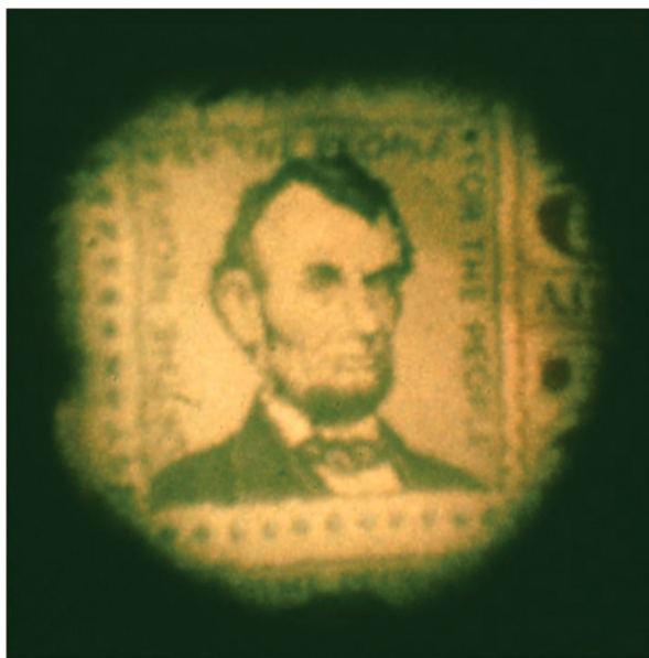
FIGURE 1. Image of Abraham Lincoln on a postage stamp taken with a camera attachment on an early fiberscope.
