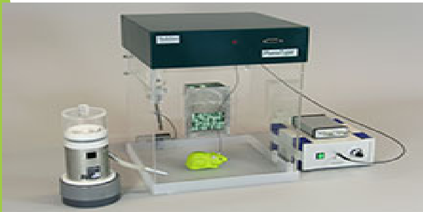
Example of PhenoTyper with pellet feeder and optogenetics
