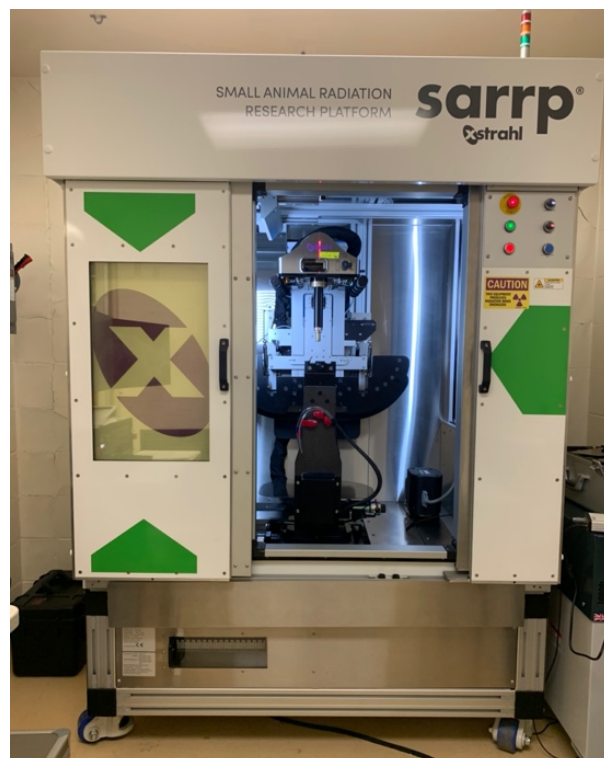
Figure 1. The SARRP system features a laser beam guide, LED cabinet lights, and live webcam views during imaging.
