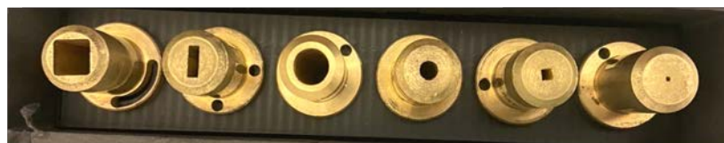
Figure 3. Several fixed size collimators are available in addition to the MVC, which allows customizable collimation.
