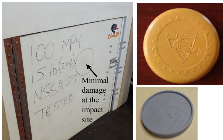
Figure 3(a) The panel that passed NSSA Category 5 tornado impact test, (b) a Frisbee, and (c) a coaster developed at UAB MPAD Center using recycled plastics.
