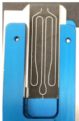
One layer CHIP system (two etched-glass plates in a sandwich)
