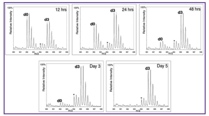
The cells are pre-labeled with leucine- $d_0$ . Leucine- $d_3$  is added to the medium and cells sampled at various times later. The peaks annotated with d0 and d3 are the triply charged peaks of the peptide VAPEEHPVLLTEAPLNPK, which contains three leucines.
