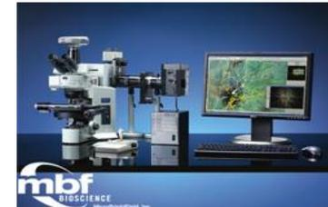
Two BX51 Olympus microscopes with Microfire optical cameras for bright field and fluorescent imaging.
