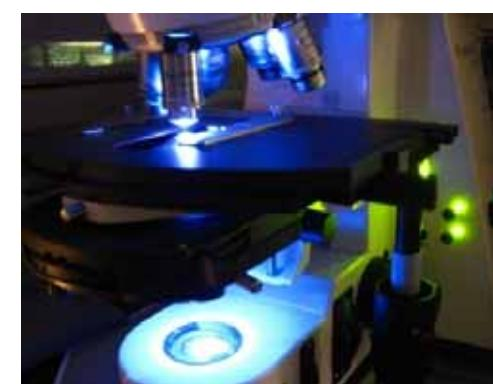
Zeiss AxioPlan2 Microscope with broad range fluorescence capabilities including DAPI, TRITC, FITC and Cy5 filters. This scope has Z-stack capabilities. The objectives are 10X, 20X, 40X, 63X and 100X. The 63X and 100X are oil immersion lenses. H. Fortinberry
