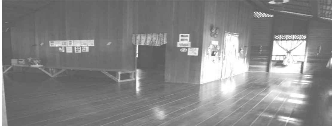
Figure 11: A hallway leading to a free area from a verandah in a Malay house from the central region. This is an example of a hallway without door or partition separating sections in the house.
